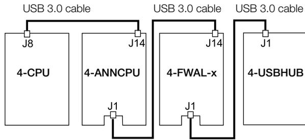
The 4-USBHUB's J1 connector may be connected directly to a 4-CPU, 4-ANNCPU, 4-NET-AD, 4-CPU-GRPH, or 4-FWAL and must always be the last device on the data bus.
